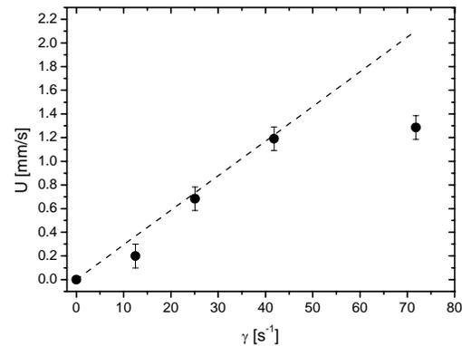
Fig. 3. The velocity of vesicle 1 as a function of the shear rate; dashed line: the theoretical results for the velocity of rigid spheres in proximity to the wall [15] (see text).
